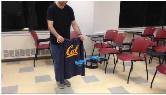
Fig. 7. Applying the Kalman Filter to the results of the object tracking algorithm, the drone rotates to keep the object in view.
